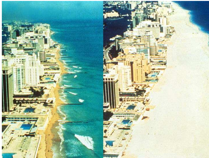
Miami Beach before (left) and after (right) the beach was widened in the mid-1970's (Houston, 2002)
