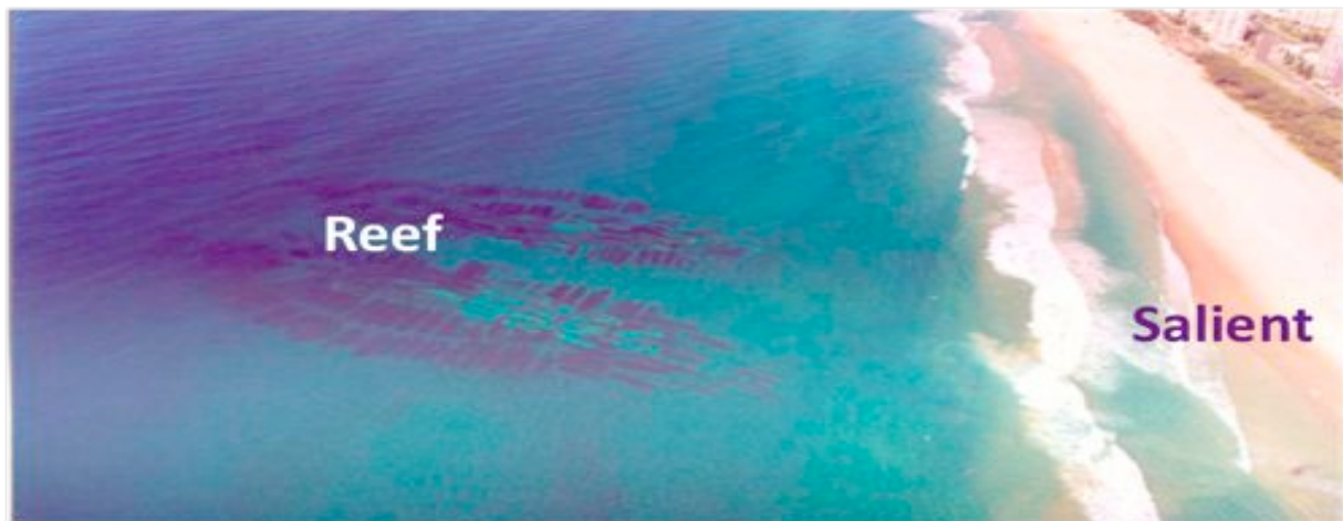
Figure 2.2 Wider beach created by the Narrowneck Multi-Purpose Reef through the formation of a salient.
