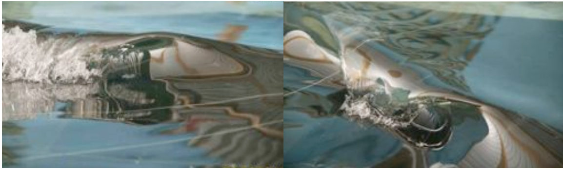
Figure 4.2 Physical modeling of a proposed Multi-Purpose Reef design in ASR's in-house wave pool facility
