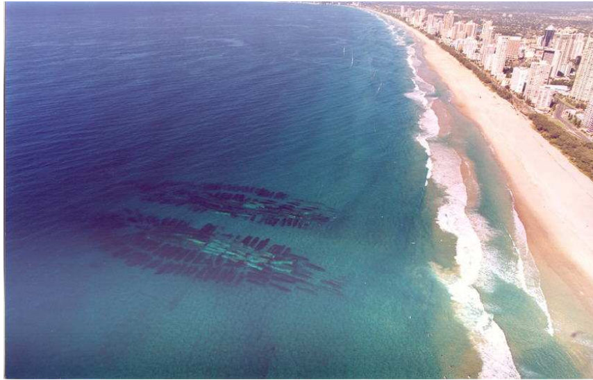
Figure 3. The view of Surfer's Paradise with the multi-purpose reef in the foreground. The lighter coloured containers had only just been deployed, while the darker containers are colonised by marine life.
